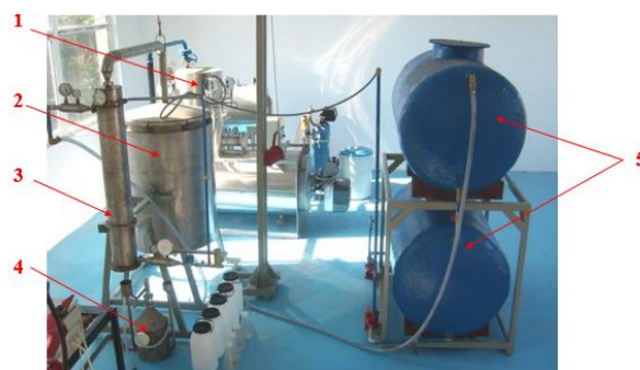
Fig. 3.1 - Steam distillation installation for medicinal and aromatic plants, IDP500
