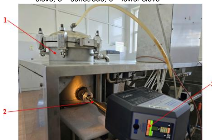
Fig. 5.8 - Aspects during the extraction process: 1 – extraction chamber, 2 – sonotrode, 3 – ultrasonic generator and control unit (Hielscher UP400St)
